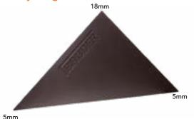
The BauderPIR FA Tapered Insulation is faced on both sides with black aluminium foil to increase thermal efficiency and is available in various thicknesses to achieve the required fall and the desired thermal requirements. The patent-pending unique ridge and valley infill boards are combined in conjunction with the Bauder FA Tapered boards to simplify the scheme and installation.
