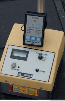
Bauder was commissioned to carry out a moisture mapping roof survey to three roof areas within the main roof with a total area of 500m². Using a Troxler 3216 Roof Reader, Bauder project surveyors were able to measure the moisture concentration within the roof structure to determine the source and extent of the water ingress.
