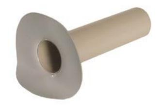
Bauder Thermoplan Emergency Overflow Outlet An extruded FPO emergency overflow outlet compatible with Thermoplan membrane.63mm diameter through wall overflow outlet manufactured in pearl white colour.
