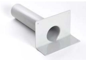
Bauder Thermoplan Rigid FPO Parapet Outlet A 90mm diameter rigid FPO parapet rainwater outlet enabling Thermoplan membrane to be welded to the flange plate. UV stable throughout. The unbacked Thermoplan membrane should be heat welded up to the aperture to ensure colour consistency on the roof.
