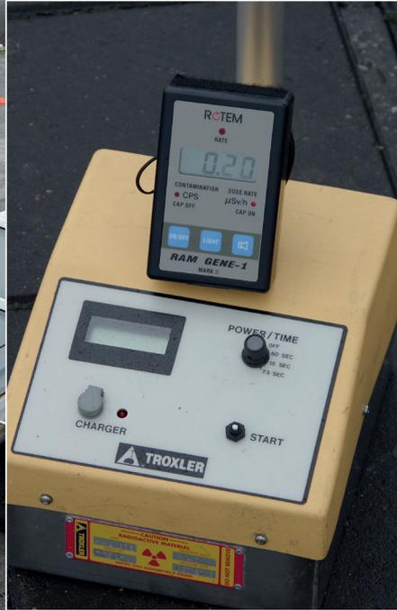
Bauder was commissioned to carry out a moisture mapping roof survey to three roof areas within the main roof with a total area of 500m<sup>2</sup>. Using a Troxler 3216 Roof Reader, Bauder project surveyors were able to measure the moisture concentration within the roof structure to determine the source and extent of the water ingress.
