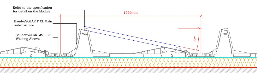
Solar Module Section - Scale 1:10
