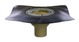
The thermal value of the rigid foam body prevents condensation from forming on the underside of the outlet body. The integrated screw down clamping ring ensures security between the waterproofing system and the outlet. It is manufactured with pre-cast studs to receive the fasteners of the clamping ring. This ensures full mechanical sealing between the outlet unit and the Hot Melt Waterproofing and Access / Protection Sheet.
