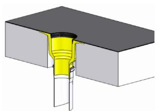
9. Place the clamping ring into position ensuring it provides a physical clamp between the Bauder Protection Sheet and outlet body. Tighten the countersunk head screws supplied with a screwdriver.
