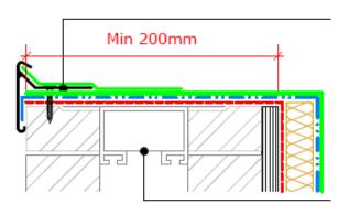
Bauder GRP water check trim to be used on parapets and perimeter kerbs wider than 200mm - must not be used on its own as a check kerb as it only has an upstand of 28mm.
