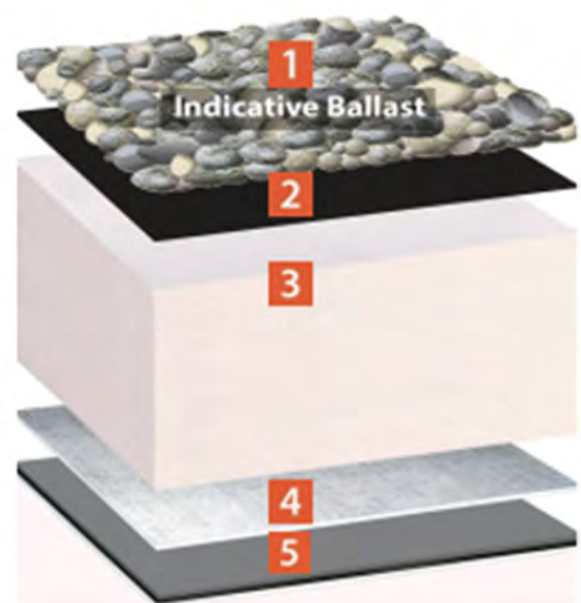
Inverted roof indicative build-up
