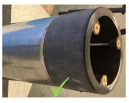
Tighten the stainless-steel screws using the mechanical seal tightening tool until the top half of the seal has expanded.
