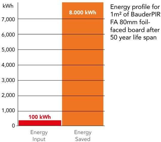
The embodied energy of our rigid polyurethane PIR insulation accounts for as little as 4% of the energy the board can save during its serviceable life. With buildings accounting for 50% of the energy consumption in Europe, the inclusion of insulation when installing new or refurbished roofs plays a significant part in reducing CO<sub>2</sub> emissions.
