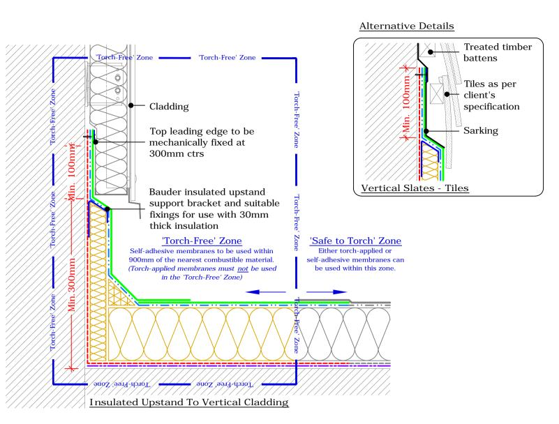
Torch-Free Insulated Upstand To Vertical Cladding Or Slates/tiles (Drg.No: D0000-00W\_201-002TF)
