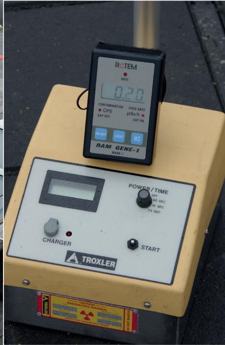
Bauder was commissioned to carry out a moisture mapping roof survey to three roof areas within the main roof with a total area of 500m<sup>2</sup>. Using a Troxler 3216 Roof Reader, Bauder project surveyors were able to measure the moisture concentration within the roof structure to determine the source and extent of the water ingress.
