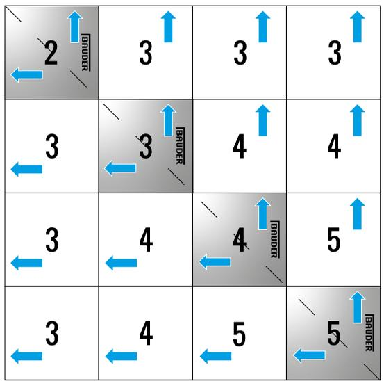
The Valley Infill pieces ensure the water can run off the roof in one direction.
