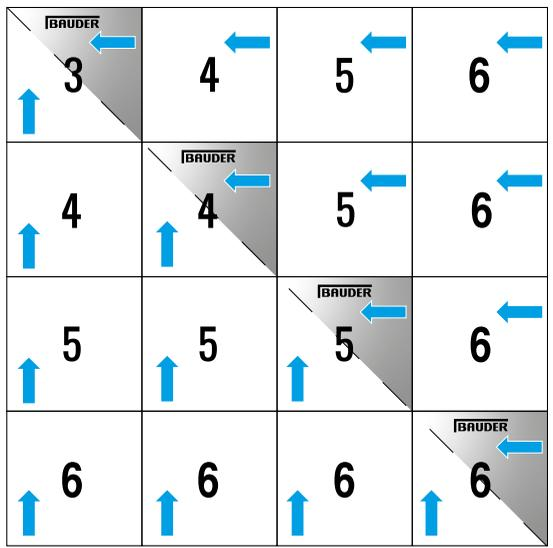
The BauderPIR FA Tapered Insulation is faced on both sides with black aluminium foil to increase thermal efficiency and is available in various thicknesses to achieve the required fall and the desired thermal requirements. The patent-pending unique ridge and valley infill boards are combined in conjunction with the Bauder FA Tapered boards to simplify the scheme and installation.
