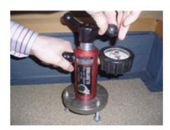
After applying a test area of LiquiBALKON or LiquiDETAIL (and recommended primer if required), cut a circular hole through the Bauder coating and upper layers of the substrate with a hole saw. Adhere 50mm dolly to the surface of the Bauder coating within the cut area and allow adhesive to cure. Carry out adhesion test with calibrated hydraulic test rig.
