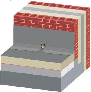
6: Mechanically fix the flange of the outlet body to the wall.
