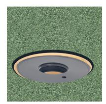
4: Lubricate the chamfered end of the overflow pipe and push into the central hole of the baseplate, a stopper within the baseplate sits at 27mm. Ensure the overflow pipe is inserted into this point.
