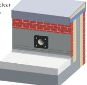
6: Install the underlayer as per specification. Cut out the underlayer to enable fitting of the overflow pipe.
