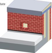
2: For insulated upstands fix the base plate to the wall at the appropriate height (determined by the finished height of the landscaping/ waterproofing).
