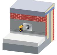
8: Prime the face plate and install the cap sheet as per specification and cut an appropriate
