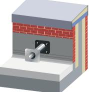
**7:** Remove and replace the grub screws with the large countersunk fixing screws.
