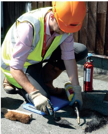
Core sampling provides localised information on the material construction of the roof's waterproofing, insulation and deck type and gives guidance on water ingress. Small sections of the roof will be effectively removed to expose the layers of the build-up down to the deck and reveal their condition with any levels of moisture recorded. Once the data has been collected for the report, the materials will be repositioned and recovered with a waterproof membrane to fully seal the examination space.
