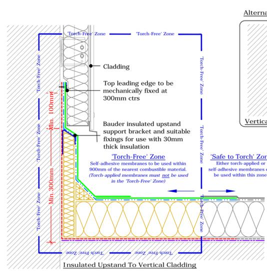
**Torch-Free Insulated Upstand To Vertical Cladding Or Slates/tiles**
