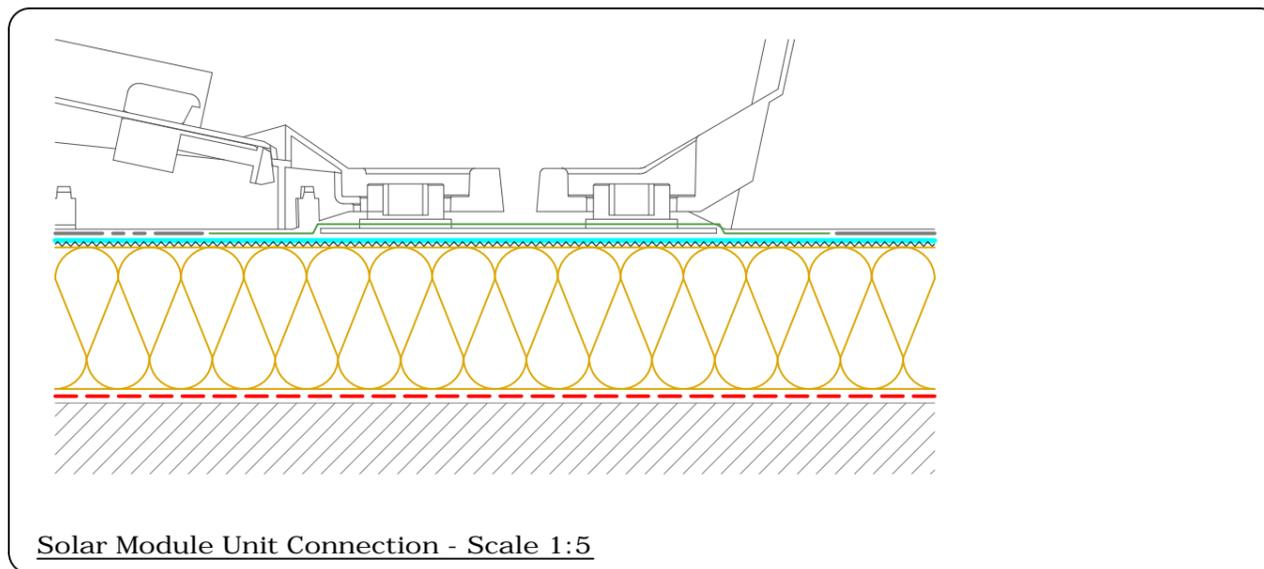
**Solar Module Unit Connection - Scale 1:5**
