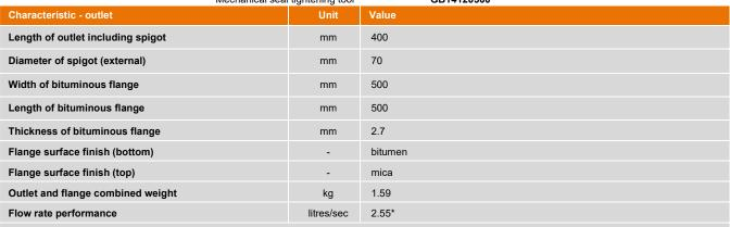
\*Flow rate performance data using a 35mm head of water (including leaf guard), based upon requirements of BS EN 12056:3:2000. Further flow rate performance data can be obtained within this document. For bespoke drainage calculation performance data, please contact Bauder Limited.
