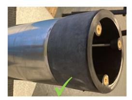
Tighten the stainless-steel screws using the mechanical seal tightening tool until the top half of the seal has expanded.
