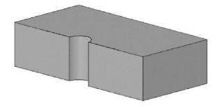
For concrete decks, the roof outlet hole (Ø 250 mm) should be pre-cast in-situ so the outlet can be installed by the roofing contractor when the waterproofing system is installed.
