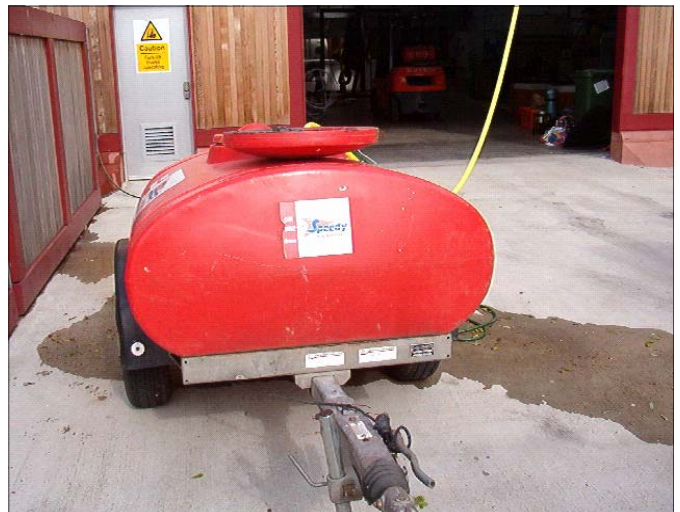
In situations where the mains water pressure is found to be insufficient, a Bowser can be used together with a pump, to provide the required pressure to roof level.
