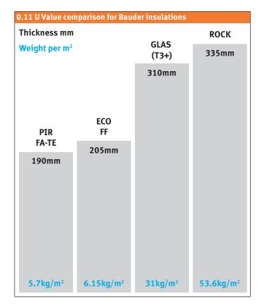
The BauderECO FF PIR foam core provides the same thermal conductivity as Bauder PIR FA-TE. The board's facings account for the differential in thermal performance between the two products.
