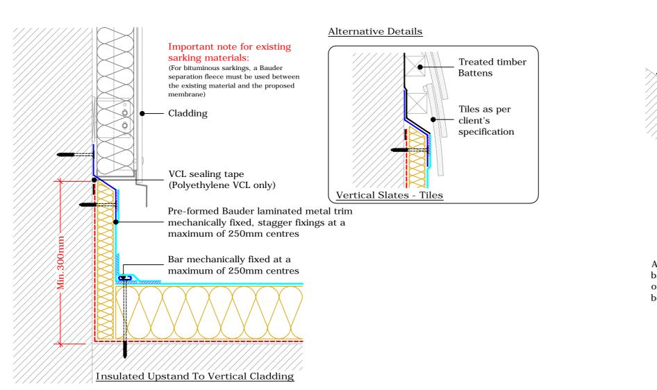
Insulated Upstand to Vertical Cladding or Slates/Tiles (Drg.No: D0100-00W\_MF\_201-002)
