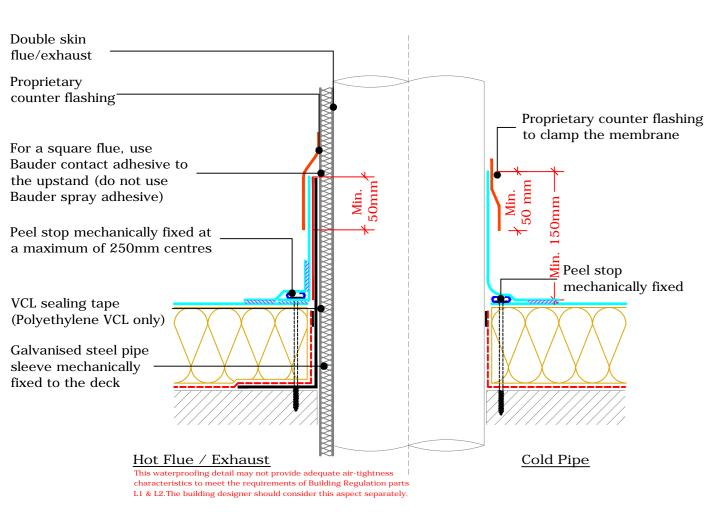
Upstand to Hot Flue OR Cold Pipe (Drg.No: D0100-00W\_MF\_007-002)
