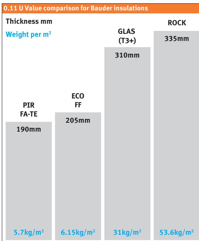
The BauderECO FF PIR foam core provides the same thermal conductivity as Bauder PIR FA-TE. The board's facings account for the differential in thermal performance between the two products.
